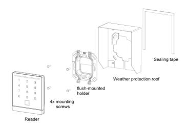
Sufficiently flexible, self-adhesive sealing tapes are included in the scope of delivery. The sealing tape is glued to the back of the weather protection roof. It prevents the ingress of water and foreign bodies.
